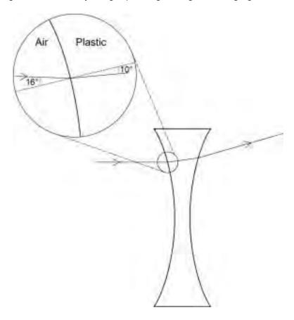
**6 (a)** Use the information in the diagram to calculate the refractive index of the plastic used to make the lens.
