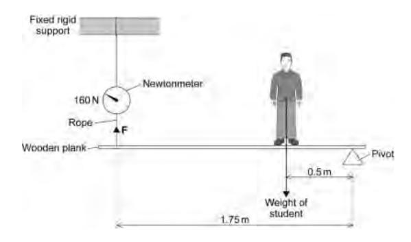
**8 (a)** Use the information in the diagram to calculate the weight of the student given by this method.
