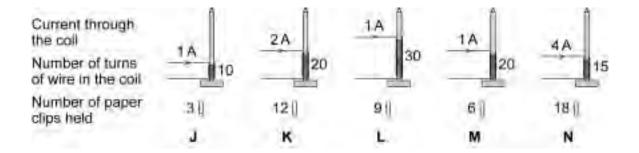
The student wants to find out how the strength of an electromagnet depends on the number of turns of wire in the coil.
